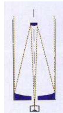
Optical cassegrain combination. We observe behind the main mirror.
