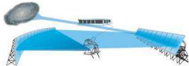
The Nançay radiotelescope and its combination of antennas allowing the reception of emissions from space. © Observatoire de Paris.
