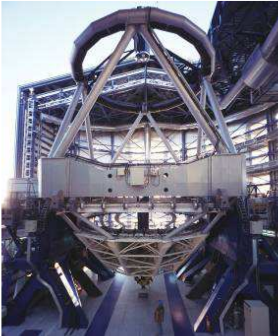
One of the four instruments of the "Very Large Telescope" at ESO-Paranal (Chile) with its 8.20m diameter mirror whose weight is 42 tons. © ESO
