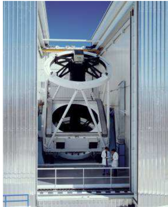
The 3.50m New Technology Telescope (NTT) at ESO-La Silla (Chile) and its azimuthal mount. © ESO.
